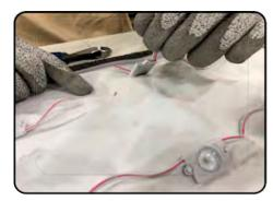
Pry off light while holding plastic pin on the back side of the fabric.
