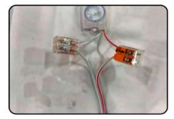
Open clamps. Match red/red and white/white wires. Insert wires in connectors and close clamps.
