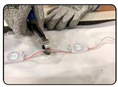
Cut wires on each side of the lights that you want replaced.
