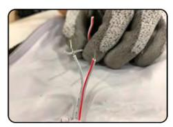
Strip the wires exposing 0.5" of the metal on both sides.
