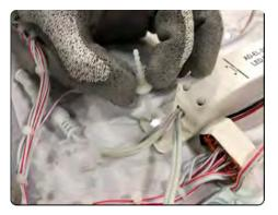
Side lock down plastic spine to secure the new power supply to the fabric.
