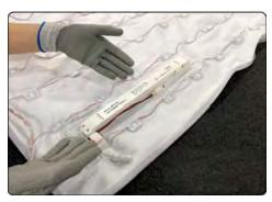
Identify the power supply that needs to be replaced. Unplug Lightblanket.
