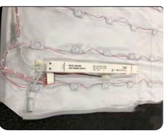
Plug-in light blanket and test to make sure new power supply works.
