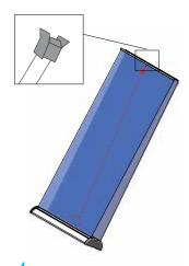
Gently lean the unit back and pull up by the toprail, and connect to top of pole.
